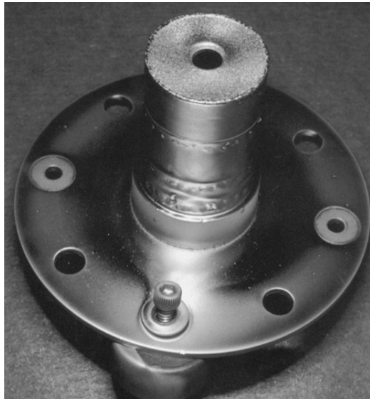
Fig. 2 EMT2 keeper after 8200 h operation.
